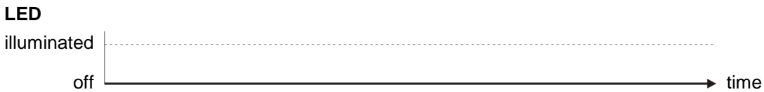
Figure 10.3: LED “Sys1” and/or “Sys2” off
