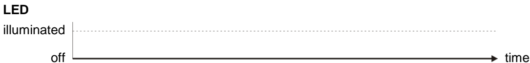
Figure 10.1: LED “PWR” off
