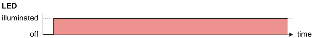
Figure 10.4: LED “Sys1” and/or “Sys2” illuminated
