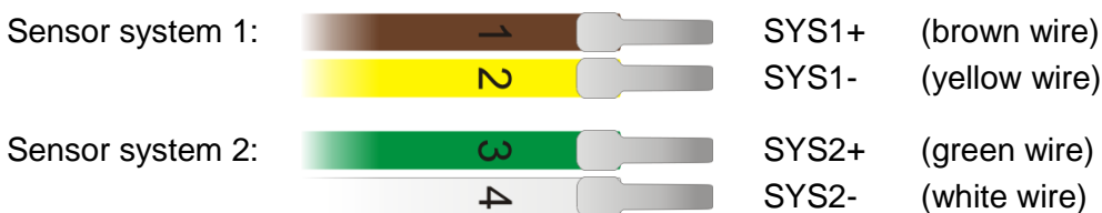
Figure 3.4: Pin assignment of the wheel sensor cable
