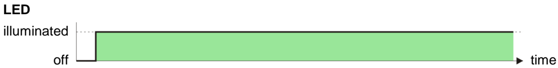
Figure 10.2: LED “PWR” illuminated
