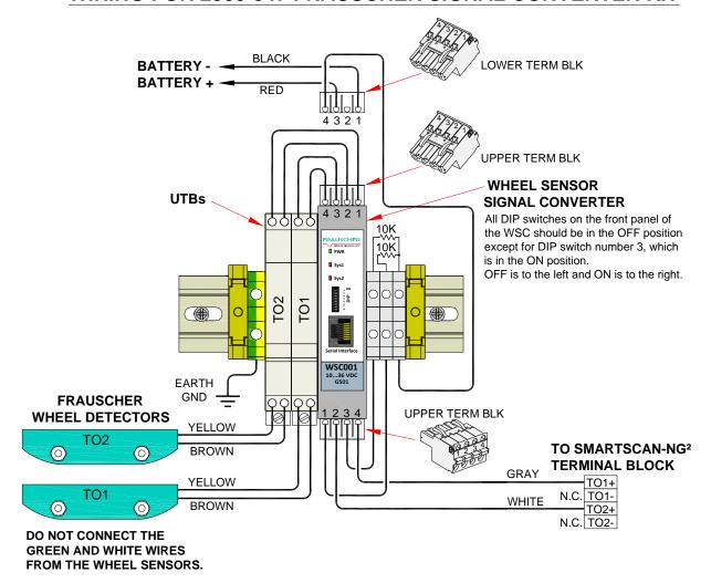
**NOTE:** This supplemental kit is applicable <u>ONLY</u> for those SmartScanNG<sup>2</sup> systems equipped with SICM Board Version 1.2 or older. Newer designs have the Frauscher interface circuitry built-in and are easily identified by a *Compatible with Frauscher Wheel Sensors* label on the cover.
