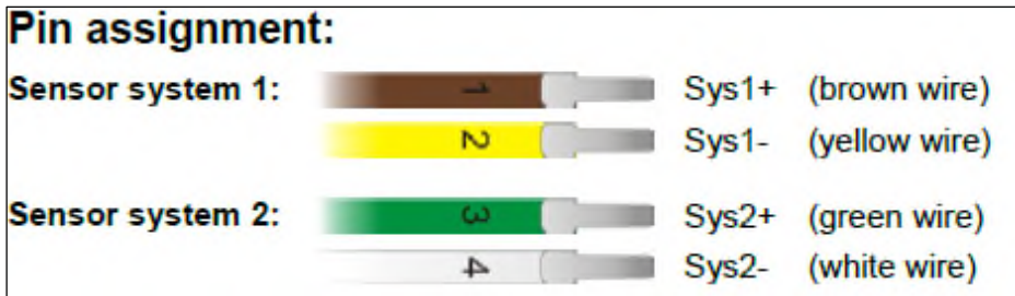
Figure 4: Frauscher Wire Color Code
